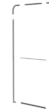
2 Add the central reinforcement tube and connect all the tubes according to the numbered system
